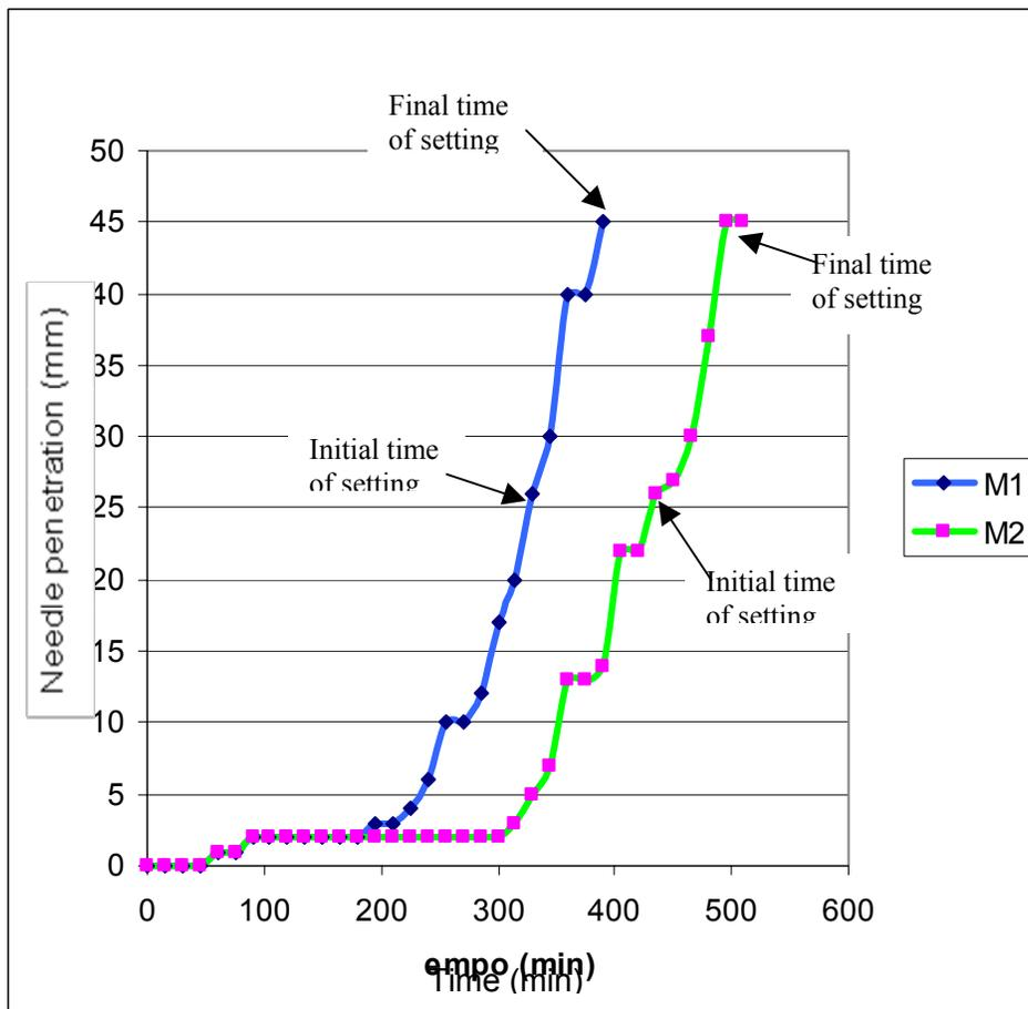
Figure 2. Comparison of initial and final setting times of mortars M1 (0% cactus powder) and M2 (5% cactus powder)
