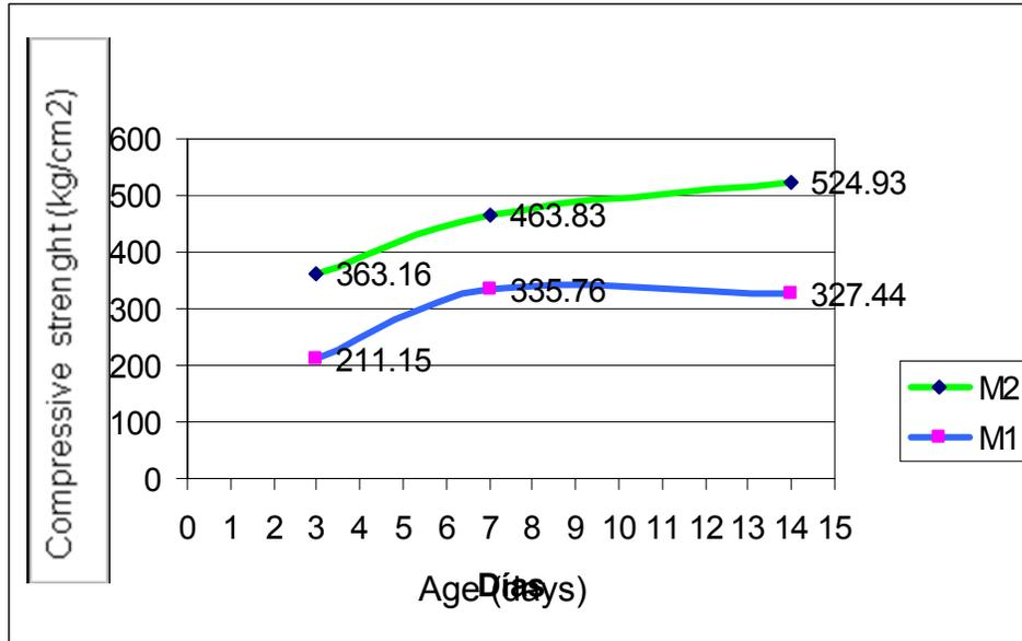
Figure 1. Compressive strengths of mixtures M1 (0% cactus powder) and M2 (5% cactus powder) at 3, 7, and 14 days of age
