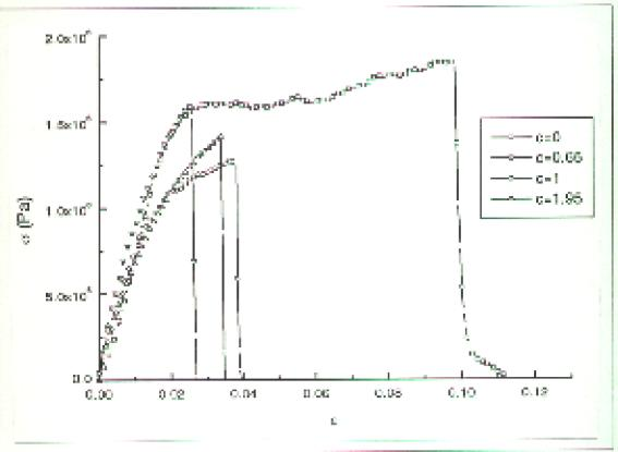
Figure 2. Stress (a) - Strain (c) Curves for Opentia few-indica Mucilage with the Ratio (c) of Mucilage to Commercial Slalood Lime
