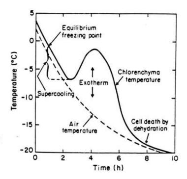
Figure 1. Generalized representation of the influence of gradual cooling of cactus stems on the chlorenchyma temperature. The stem supercools below the equilibrium freezing point, then an exothermic reaction occurs as ice crystals form extracellularly, followed by continued cooling accompanied by water distilling out of the cells and being incorporated into the growing crystals, eventually leading to the concentrating of cellular contents and death by cellular dehydration.
